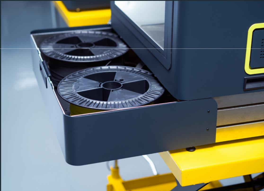
The integrated Material Station can fit two spools of filament up to 2,5 kg each to maintain continuous work for a long period of time. This means bigger models are possible to print at once.
